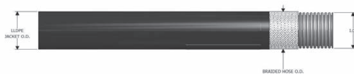
Figure 1 - Extruded Hose Dimensions
