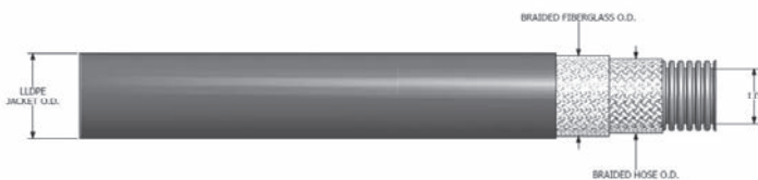
Figure 1 - Insulated Extruded Hose Dimensions
