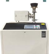
Cryogenics and Vacuum Jacketed Assemblies are Helium Leak checked to 1 x 10-9 std. cc/sec
