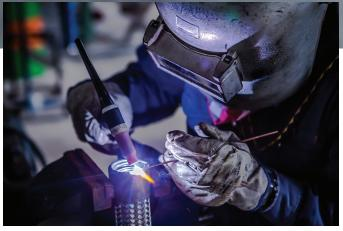
Omegaflex welders and Omegaflex welding procedures are qualified to Section IX of the ASME Boiler and Pressure Vessel Code. Omegaflex hose assemblies are qualified to ISO-10380:2012
